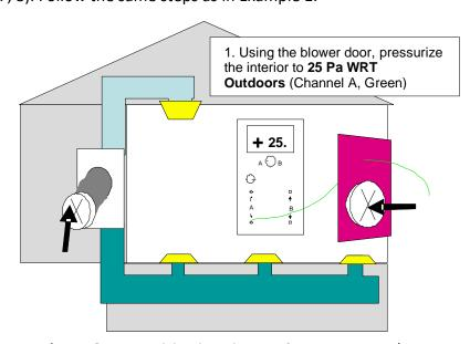
Figure 6: Pressurizing interior to +25 PA WRT outdoors
