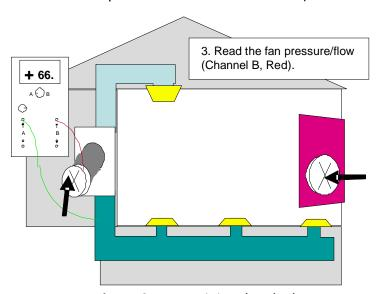
Figure 8: Determining duct leakage
