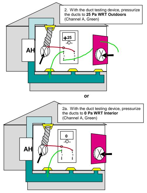
Figure 4: Pressurizing ducts to +25 PA WRT outdoors, or 0 PA WRT indoors (duct testing device hooked up to largest return duct, inside the pressurized zone of the house)
