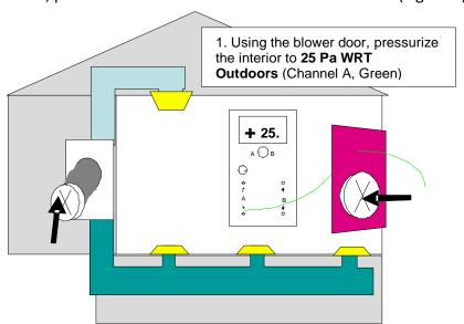
Figure 3: Pressurizing interior to +25 PA WRT outdoors
