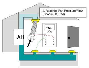
Figure 2: Determining duct leakage
