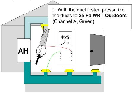
Figure 1: Pressurizing the duct system
