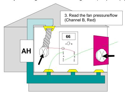
Figure 5: Determining duct leakage
